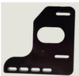
Fasten the focus motor to the focus motor mount plate. Fasten the belt drive pulley to the focus motor. Look at the motor mount block. The dovetail slot on the bottom allows it to slide on to the main dovetail plate side rail. Slide the block on to the rail. Don't attach the motor plate to the block because you don't yet know which holes to use.
