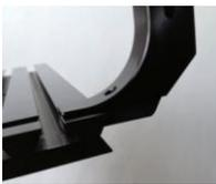
Slide the toe of one of the risers into the cross slot. It doesn't go in far, the end of the riser dovetail pin only goes in so it is even with the inside edge of the first rail. Gently snug the set screw in the bottom of the dovetail plate so it just holds the riser in place but you can still slide it a bit if you want. Repeat with the other side.
