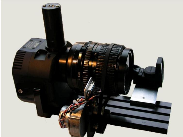
The camera mounting bracket makes extensive use of sliding dovetails. The dovetail joint gets immense strength from a trapezoidal pin trapped in a slot. The internal flats of the dovetail joint make the joint self aligning, intrinsically orthogonal, and very rigid. Sliding dovetails make this camera mounting bracket enormously adjustable.
