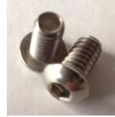
**NOTE: You must not use a screw or bolt longer than 1/2 inch.** The supplied button head screws are 1/2 inch long. If you lose one of the supplied button head screws and replace it, make sure that you don't get one that's too long. (Using a screw or bolt that is too long can damage your camera because the long bolt can be turned with such force that it can punch through the thin aluminum that forms the base of the camera's tripod socket.)
