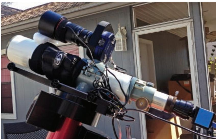
Image 2 - An early, less-successful configuration attempted to support the 200-mm lens with a bit of foam.
