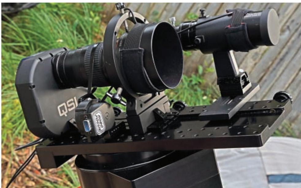
**Image 7 - The completed Wide-Field Dream Machine incorporates Telescope Support Systems camera-lens mount ring, Starlight Instruments QSI-camera mounting hardware, a Starlight Instruments-sourced motor-focus system based on a design by David Ellison and a Canon lens.**
